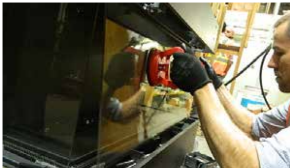
Handle front panel with supplied vacuum clamps
